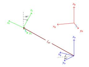
$$C_{c}^{a} = C_{b}^{a}C_{c}^{b} = R_{z,50^{\circ}}R_{y,-30^{\circ}}$$
