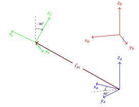
$$\begin{split} C_b^a &= R_{z,50^\circ} \\ C_c^b &= R_{y,-30^\circ} \\ \vec{r}_{ab}^a &= \begin{bmatrix} 0 & 0 & 2 \end{bmatrix}^T \\ \vec{r}_{bc}^b &= \begin{bmatrix} 3 & 0 & 0 \end{bmatrix}^T \end{split}$$
