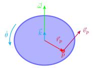
From mechanics, linear velocity  $\vec{v}_p$  of point is
