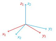
Fixed Axis Rotation Rotate about z<sub>1</sub>
