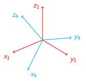
Fixed Axis Rotation Rotate about *x*<sub>1</sub>
