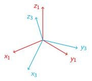
Fixed Axis Rotation Rotate about y<sub>1</sub>
