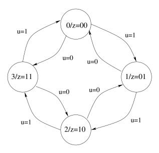
There are many ways to design state machines using AHDL. Here are one design for the two-bit up-down counter:
