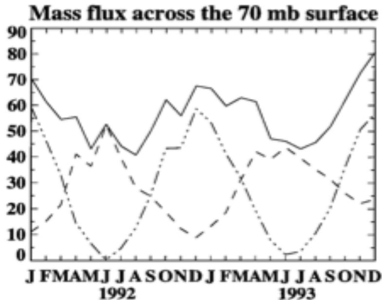
**Figure 14.** Time series of mass flux across the 70-hl surface in units of  $10^8$  kg/s computed from the radiative-derived stream function. Solid curve is the net upward tropic flux; dotted-dashed curve is downward flux into the northern hemisphere; dashed curve is downward flux into the southern hemisphere.
