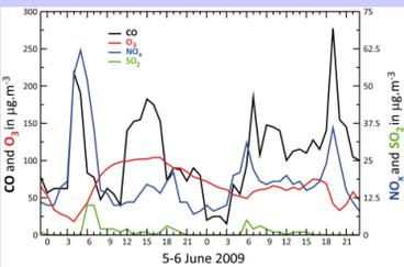
Fig. 2 (above right): Temporal variability: O<sub>3</sub> (red), CO (black), NO<sub>x</sub> (blue), SO<sub>2</sub> (green), measured over period 5–6 Jun 2009 at Reims, France [x axis: hr; y axis: concentration (µg m<sup>-3</sup>)]. © Copyright 2012, American Meteorological Society (AMS) Lahoz *et al.* 2012 (BAMS).
